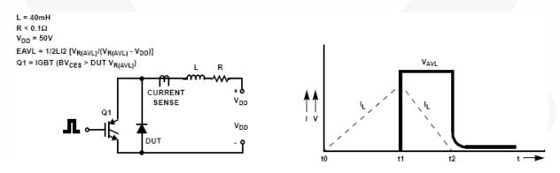
Figure 2. Unclamped Inductive Switching Test Circuit & Waveform
