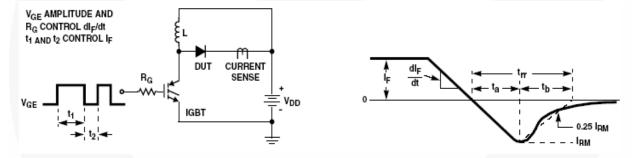
Figure 1. Diode Reverse Recovery Test Circuit & Waveform
