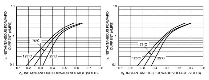
Figure 1. Typical Forward Voltage
