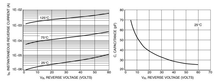
**Figure 3. Typical Reverse Current**
