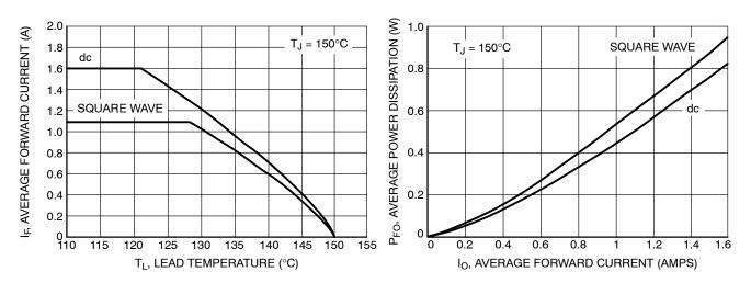
Figure 5. Current Derating - Junction-to-Lead
